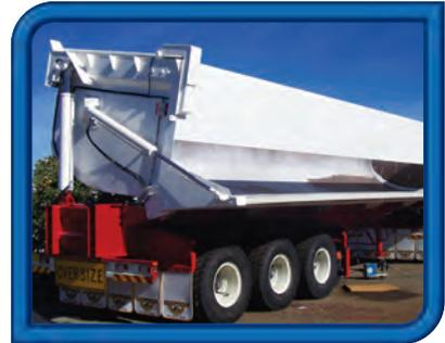
Heavy duty double acting hydraulic door, pivots made from 41/40 bar and bush, cylinders mounted on end walls so no internal obstruction to cause product build-up or hanging.
