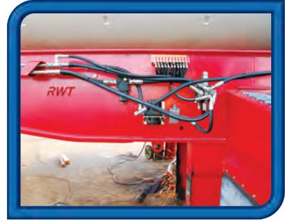
Unique 3 in 1 Solid Aluminium Control Valve. External hydraulics for easy access and maintenance. Treated hydraulic lines for durability and long life.
