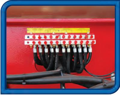
Remote grease points for ease of maintenance and safety requirements.
