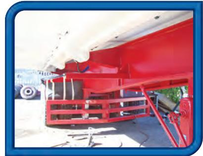
Fully welded high tensile Domex chassis with one piece web full width frame to protect the 385/95/R25 tyres and under carriage.
