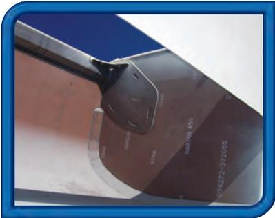
Large radius side wall to eliminate hang-up. 10mm Hardox 450 floor, walls and door 8mm Hardox 450 liner plate corners and joins braced for added strength.
