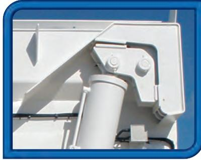
Floating top lift cylinder mount to minimise unnecessary movement and prolong seal life.
