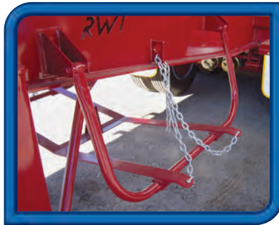
■ Swinging dual spare type carrier.
