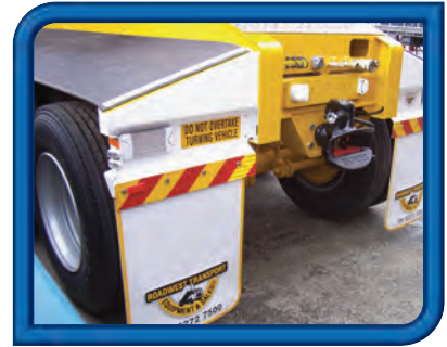
■ Rubber mud flaps front and rear of suspension, spring tensioned rubber guards over tyres, rubber protection flaps over rear coupling.
