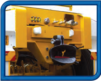
■ Fabricated steel bracket to rear with air, electrical, hydraulic couplings and Ringfeder.
