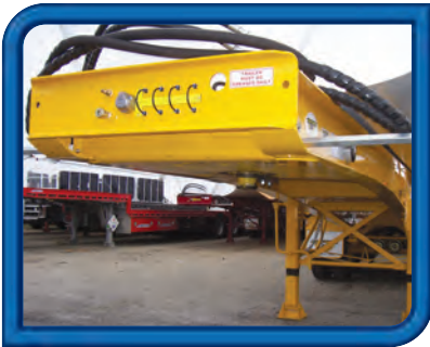
■ Strong lead-in plate and front bolster protects air, electric and hydraulic fittings.
